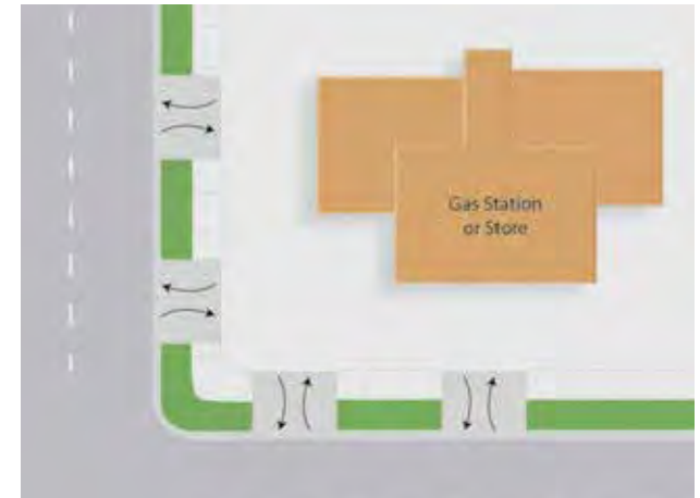
Corner with many wide driveways (Credit: Michele Weisbart)
